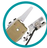
Runner chuck EM (Proximity sensor-attachment/ detachment claw)
